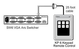
Figure 1 — Typical KP 6 application (with 9-pin D-sub connector)
